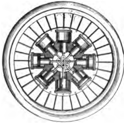
FIG. 21. —Bergman's Steam Motor Wheel. A number of steam cylinders are arranged within the hollow hub of the wheel, so as to act on a common crank on the axle. The action is on the plan of a compound engine, the steam being exhausted at low pressure.
